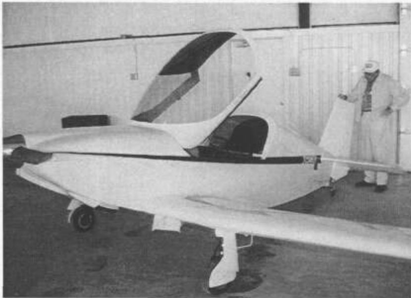
The only premade component on the Betchan KR-2 is the Dragonfly plexiglas canopy. Additional framework and skirting, plus forward hinge mechanisms, were crafted by the builder. KR's small size shown evident.
