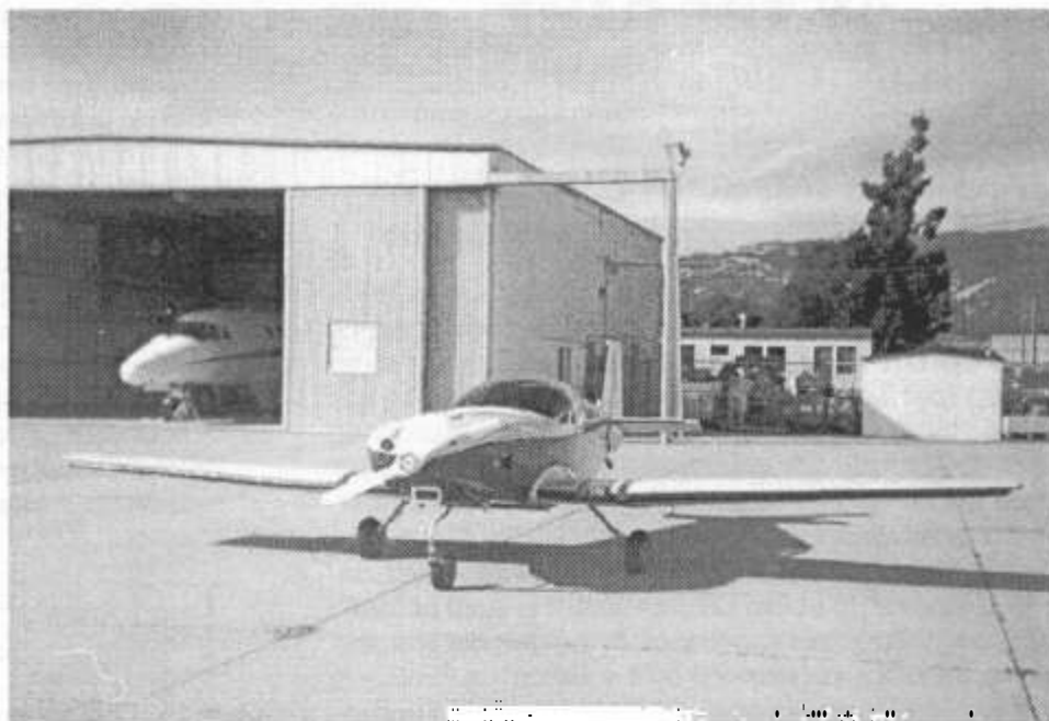
Subaru EJ-22 is neatly cowled in the Vogt KR-2S. The paint scheme includes a beautiful blue-green on the lower portion of the fuselage along with a subdued stripe that makes the 2S look even longer and leaner than it already is.
