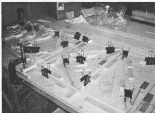
Flexible wood strips, combined with metal spring clamps, secure fuselage gusset blocks during epoxy application.
