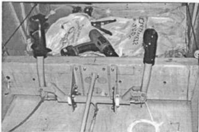
Main spar forward attachment for spar compression brace. Unit mounts on aircraft centerline and does not interfere with dual control stick assembly. Note details of both components.
