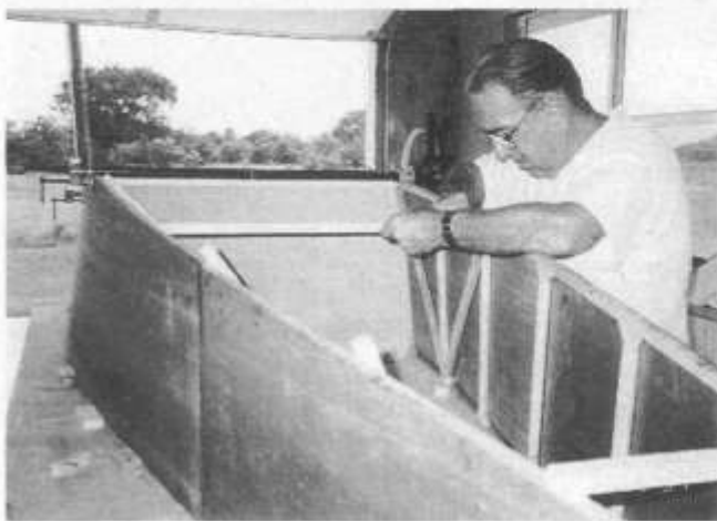
With fuselage solidly held in place by formers, cross member installation is done at a more relaxed pace.
