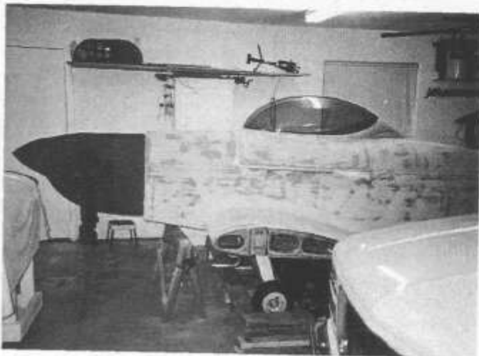
A cardboard cowling profile is utilized to check outline from spinner to firewall thereby saving later surprises.
