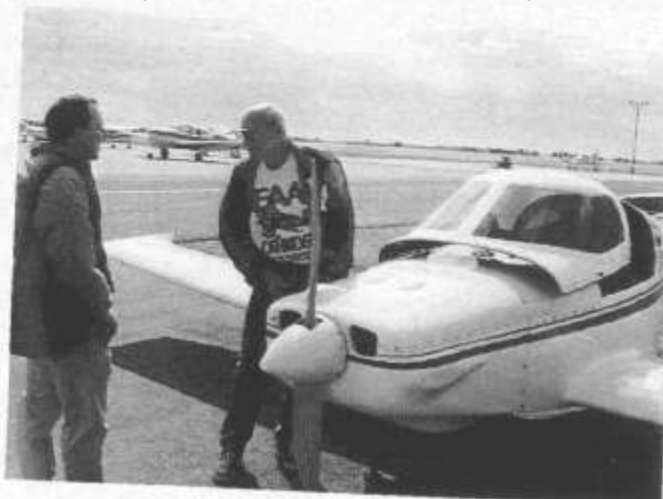
Stealthy-looking canopy on the Dennis Pointer tri-gear KR-2.
