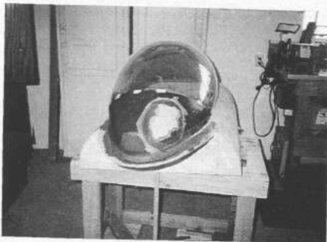
Accidents will happen. Damaged during storage, the canopy is repaired with fiberglass both inside and outside the frame. Common drywall patch fills void.
