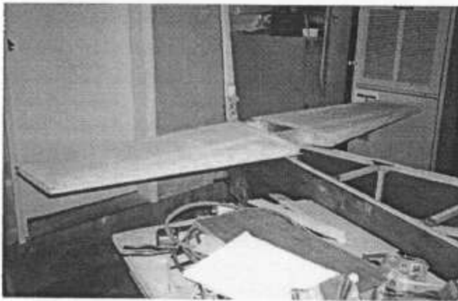
Plywood-skinned horizontal stab in position.
