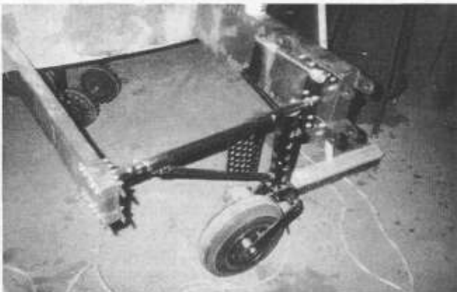
Main gear as is attached to wing's center section spars. Note the pneumatic operating cylinder position.
