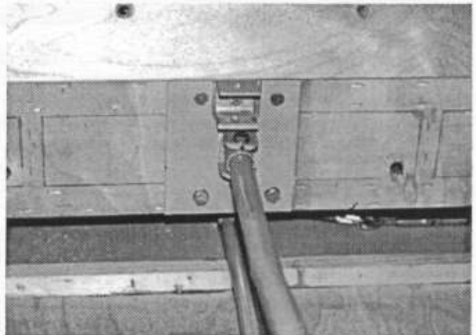
Aft spar attach detail for spar compression brace. Empty u-channel is for attaching the rear tube of the seat sling.
