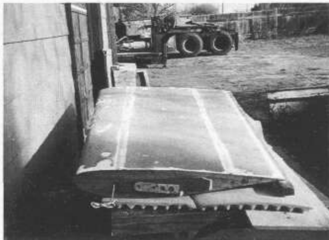
Traditionally constructed KR wing with shaped foam, filler and fiberglass demonstrates Jim's craftsmanship.
