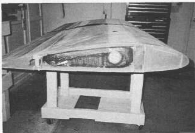
Fuel tank nested in wing and secured in wooden cradle epoxied to spars. Also note the wheeled work cart and Stan's obscenely clean shop.
