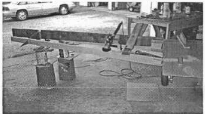
Overall view of KR wing spar beveling operation. Spars are properly spaced by tip rib and supported from below with blocking to help hold position during grinding ops.
