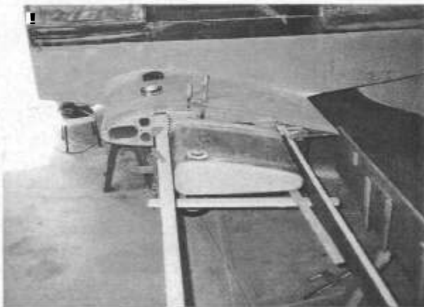
Custom fiberglass wing tanks undergoing trial fitting in the Mello KR project. Stan relates his learning curve is near vertical at this point in the construction process.
