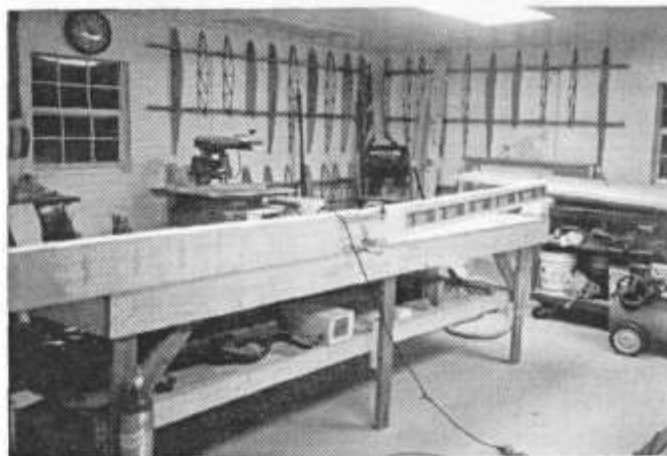
Setting dihedral in the KR's main spars. Positioning the Spar Attach Brackets is a critical construction step. Bob's sturdy work table insures accuracy.
