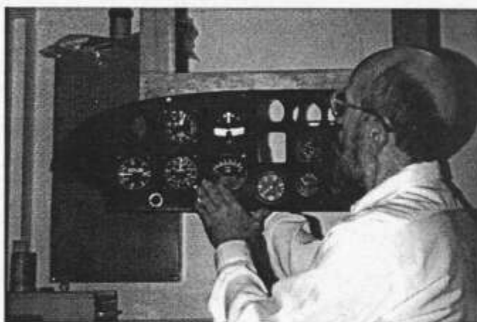
Initial fit up of instruments was done with panel attached to ceiling-suspended jig. Good idea is easy on the back.
