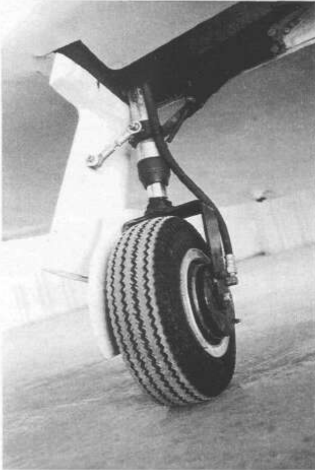
Japanese Hodaka motorcycle front forks are recycled into landing gear struts on the Betchan KR-2. An old Buick also provided some retraction components.
