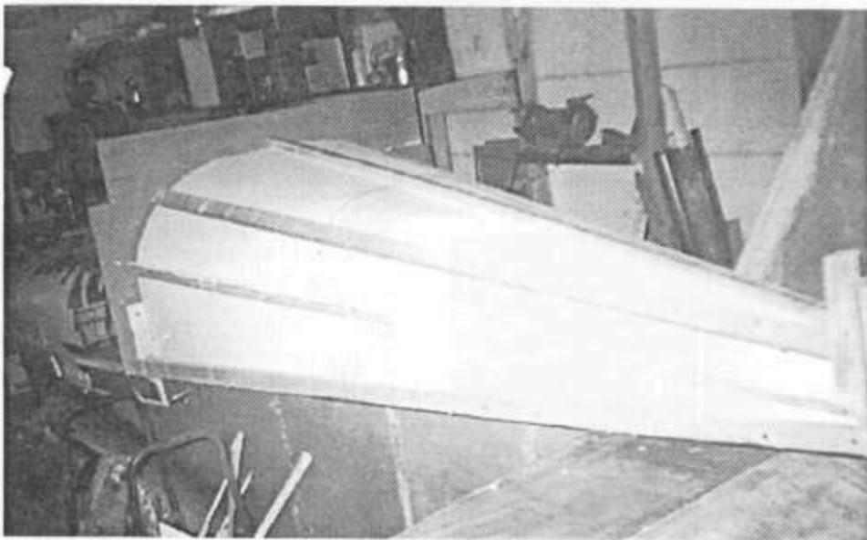
Scratch-built aft deck utilizes formers and stringers to maintain position of structural foam prior to application of fiberglass skin.
