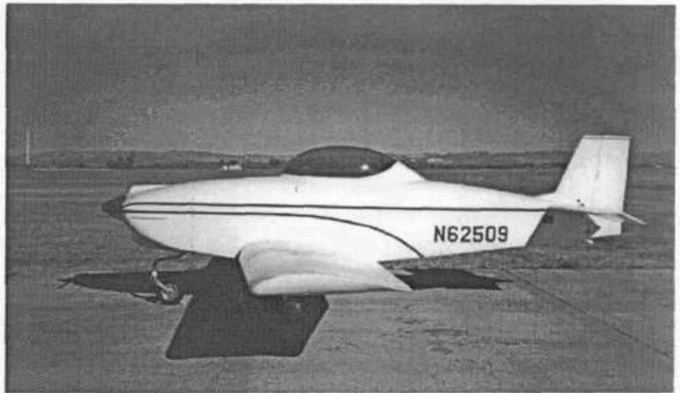
Bet your first guess was wrong! it's a custom KR-2 built by Stan Mello of Paso Robles, California. The Dash-One canopy, tri-gear, and lowered aft fuselage deck creates the unique side view.
