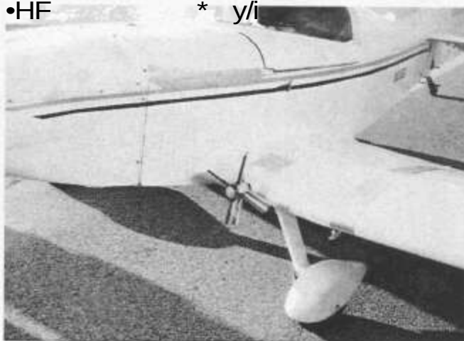
Access to the 8 amp, wind-driven alternator in Randy Clark's KR2 is through an aluminum access plate on top of the wing's center section.
