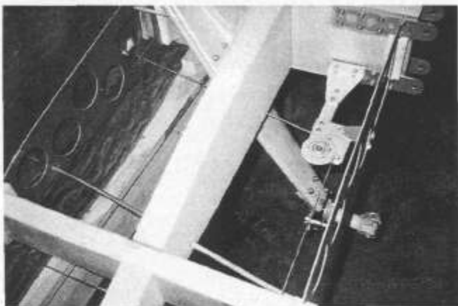
Aileron cable bracket modified to clear gear.
