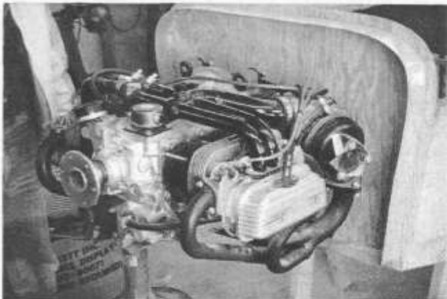
A Hapi 1835cc Volks with an exhaust-driven turbo will power the completed Eason KR-2.
