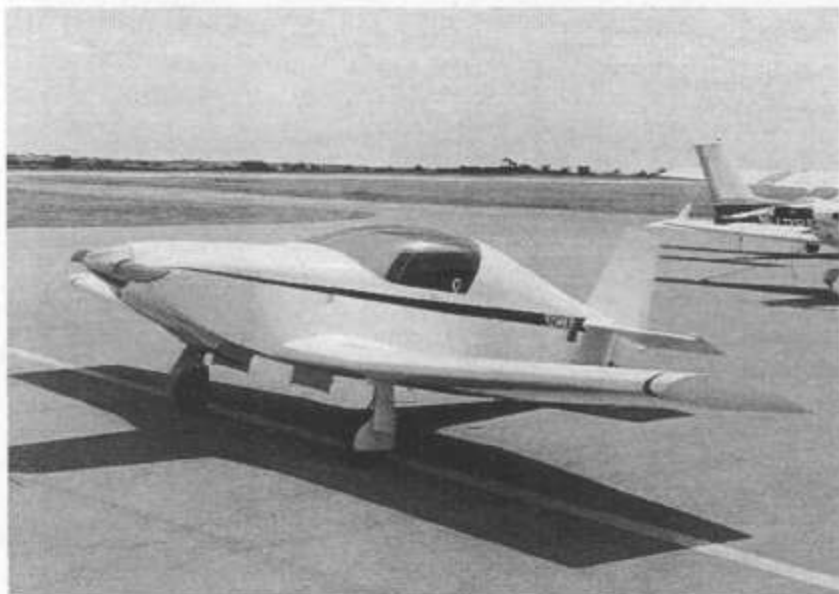
Beautiful hand-crafted cowling blends the lines of the KR-2 from its polished spinner to the forward hinged Dragonfly canopy.
