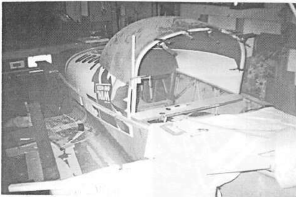
Cockpit canopy goes through an initial test fitting with a mock-up of the aft deck.
