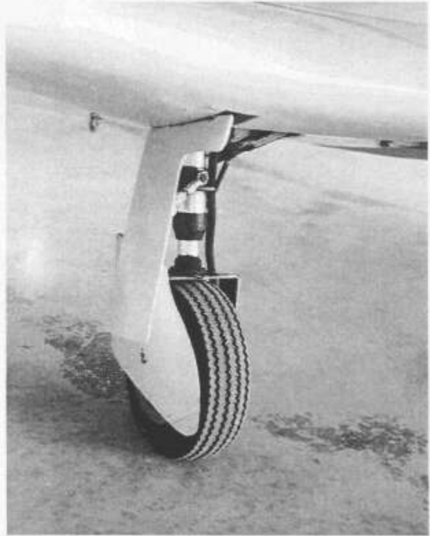
Two-piece, articulated main gear door covers, when combined with inner doors, create a major component of the drag reduction features on N250KB.
