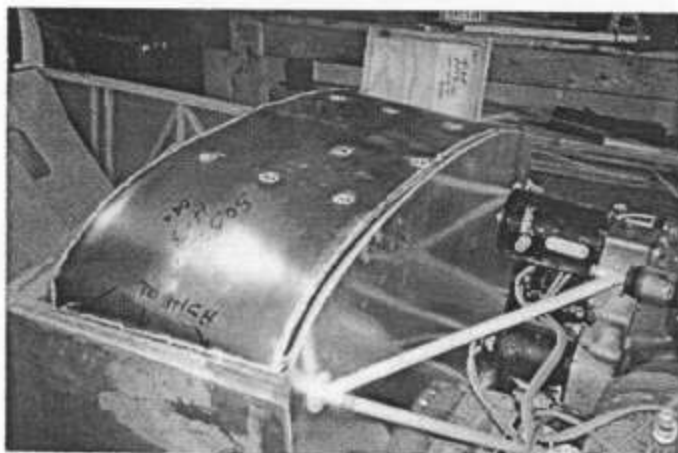
KR2 fuel tank is fabricated of .040 5052 aluminum.
