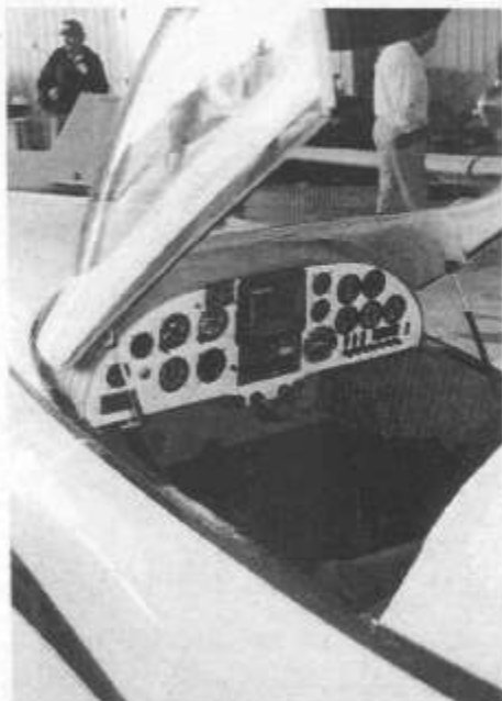
A deluxe Day-VFR panel includes a kit built RST 720 NavCom. GPS on top.
