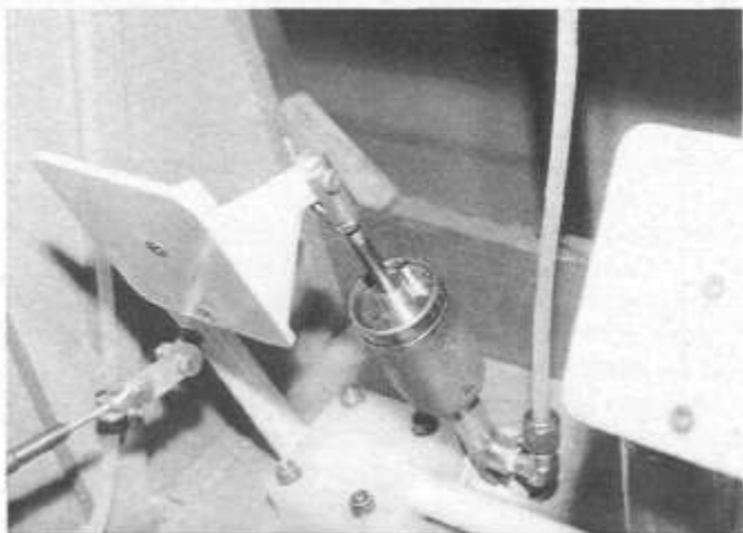
Hydraulic brake cylinder modified with brass fitting for simple and clean servicing of brakes.
