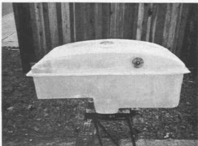
Buckner's bladder-buster 21 gallon header tank No mention in his builder's report of a relief tube!
