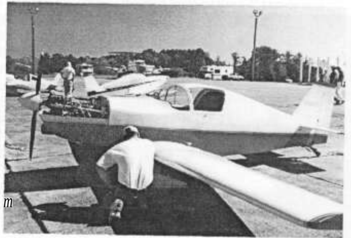
This belt redrive, Subaru powered KR2 also featured a very cleanly executed fixed windscreen canopy. Much interest in this aircraft. Troy Pettaway's KR in backgrnd.
