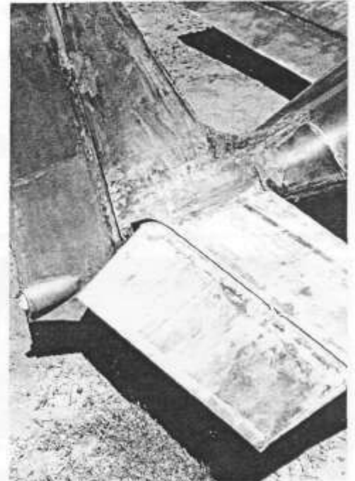
Careful attention to tail surfaces juncture will aid performance. Note nav light.
