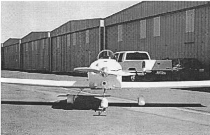
Coming at you, the Mello KR2-M displays its low frontal area, KR-1 style cockpit canopy and multiple drag reducing fairings. Very sleek.
