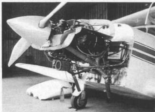
True to form, Bob made his own intake and exhaust systems, carb heat box, baffles and modified the Posa to provide inflight mixture control.
