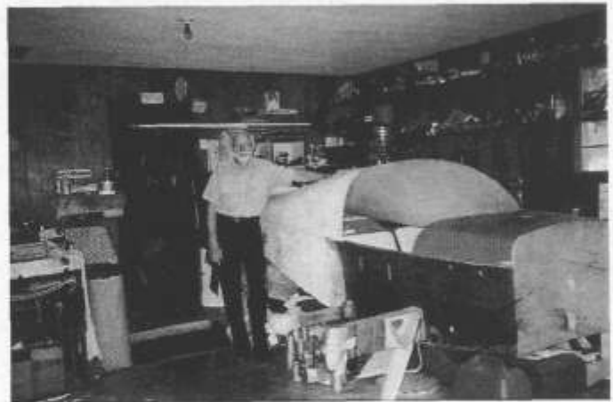
Whiskers John Gregory with his stretched T-Tailed KR-2. With fixed mains and a retractable tailwheel, the Revmaster 210DD should punch nice holes in the sky.
