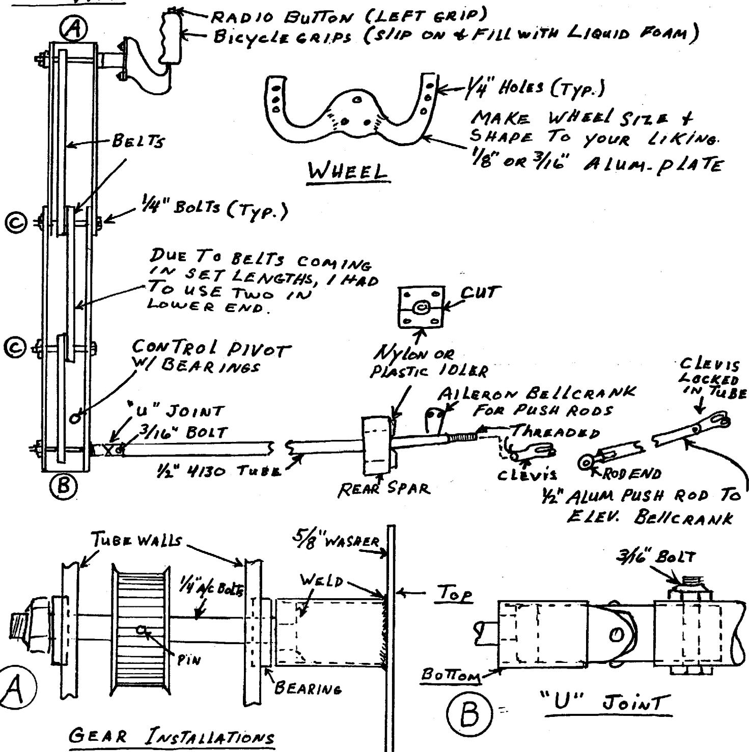
All gears are the same size except the bottom gear so I could have more "feel" on the ailerons, so I used one 1.4 larger.
