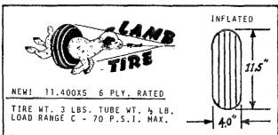
This tire fills the size gap between the 500x5 aircraft tire and the 3.40-3.00x5 go-kart tire. Looks like a scaled-down 500x5. Fits KR-1 & 2's and is recommended by Burt Rutan for the variEZE and longEZE. Also fits most other experientals using 5 inch rim's.
